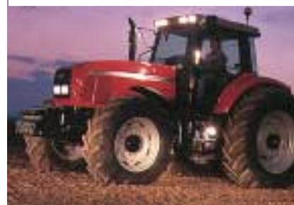
Above: Additional front, rear and footstep mounted work lights are available
